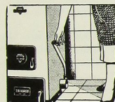
Simple movement of lever and boiler is declinkered in two seconds without dust or loss of heat.
